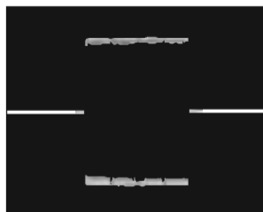
HP 8340B/8349B/83554A Pulse Performance at 36 GHz. Pulse width = 5 \mu s.
